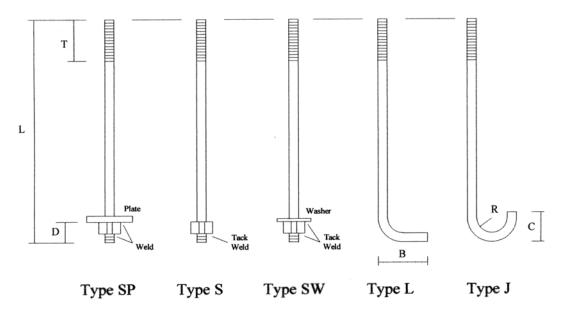
Construction Anchors has the ability to provide custom shape anchor bolts cut, threaded and bent to your exact specifications. We can in-house fabricate anchor bolts from 5/8" to 1/2" diameters.
