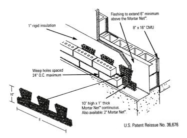
Mortar Net is the leading mortar dropping collection product providing the solution for clogged weep holes in brick cavity construction. Featuring a patented design and 90% open-mesh weave, Mortar Net catches and suspends mortar droppings and other debris above the weep holes. Mortar Net prevents the mortar from forming a barrier against necessary flow, allowing for the free migration of moisture from the wall to the weep holes.
