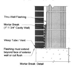
Mortar Break is .8" thick and designed for use in 1" cavities. **Size:** 10" x 50 ft. rolls.
