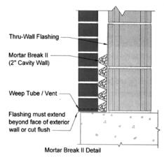
Mortar Break II is 1.5" thick and designed for use in 2" cavities.
