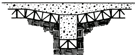
Typical interior grade beam and slab
